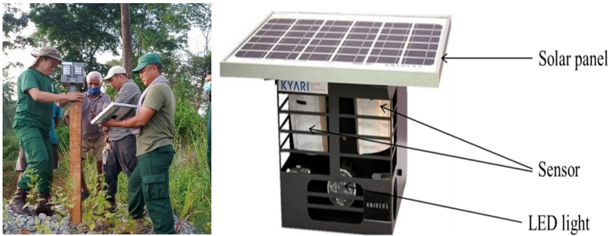
Figure 40: Animal intrusion detection and repellent system (ANIDERS).
